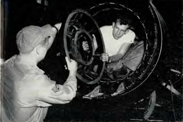
Left, Capt. Bert E. Bookout, Jr., Maintenance Officer for the 538th FIS, receives the Air Force Commendation Medal from Major Thomas H. Cribbs, new commander of the squadron. Center, SSgt. Arthur J. Smith and A/3C Raymond A. Kramer install the burner ring of the F-104 interceptor. Right, SSgt. Arthur J. Smith checks the gages during engine runup while preflighting a Starfighter.
